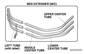
7. Install the strap to the middle tube of the right tube. Slide three center tubes into the right tube using the coated area as a guide for depth of insertion.
