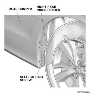
Install one spring nut into the right rear inner fender hole.
