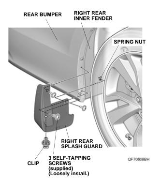
Secure the right rear splash guard with the three self-tapping screws in the order shown below.
