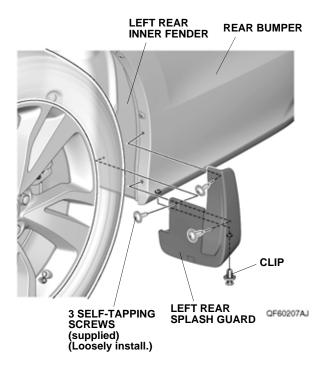
Secure the left rear splash guard with the three self-tapping screws in the order shown below.
