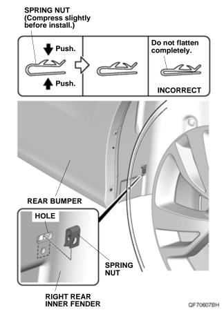
17. Loosely install the right rear splash guard on the rear bumper and spring nut with three self-tapping screws and clip.
