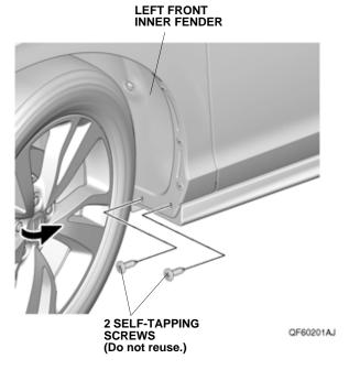
Remove the two self-tapping screws from the left front inner fender. 3. Using a pushpin, pierce the center of the two clips on the left front inner fender.
