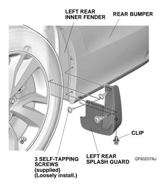
11. Secure the left rear splash guard with the three self-tapping screws in the order shown below. NOTE: Make sure there is no gap between the left rear splash guard and the bumper. If there is a gap, loosen the self-tapping screws, hold the splash guard against the bumper, and retighten the screws.
