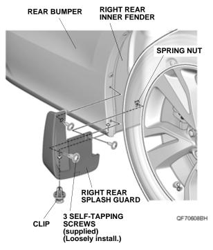
18. Secure the right rear splash guard with the three self-tapping screws in the order shown below.
