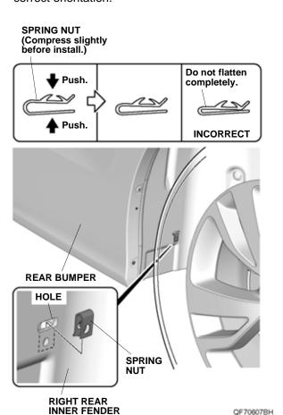
17. Loosely install the right rear splash guard on the rear bumper and spring nut with three self-tapping screws and clip.
