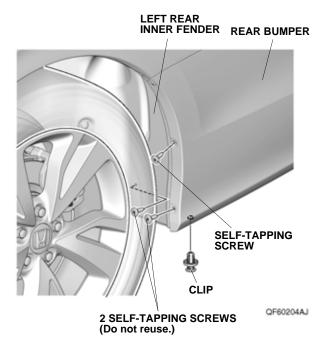
Locate the recessed mark. Using a pushpin, pierce the rear bumper at the recessed mark.
